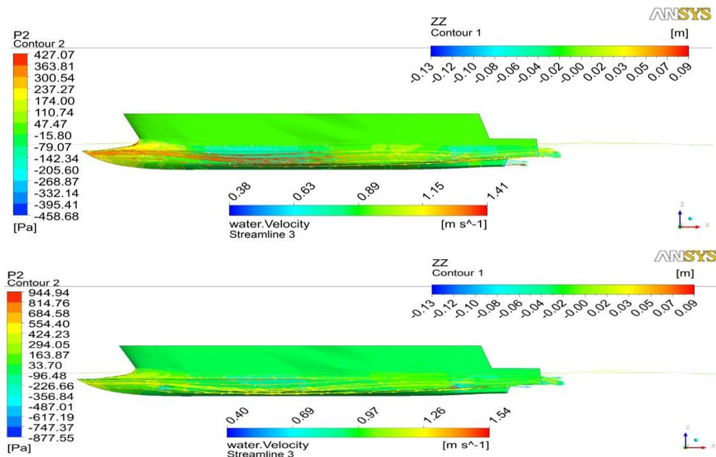
Figure 6: Pressure distribution contour plot of the Semi-SWATH at  $Fr = 0.34$  and  $Fr_H = 1.0$  for the deep water condition: (top) without fin stabilizers, (bottom) with fin stabilizers ( $\alpha = 0^\circ$ )
