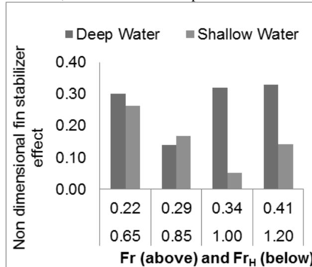
Figure 5: Comparison of the fin stabilizer effect between deep water and shallow water conditions
