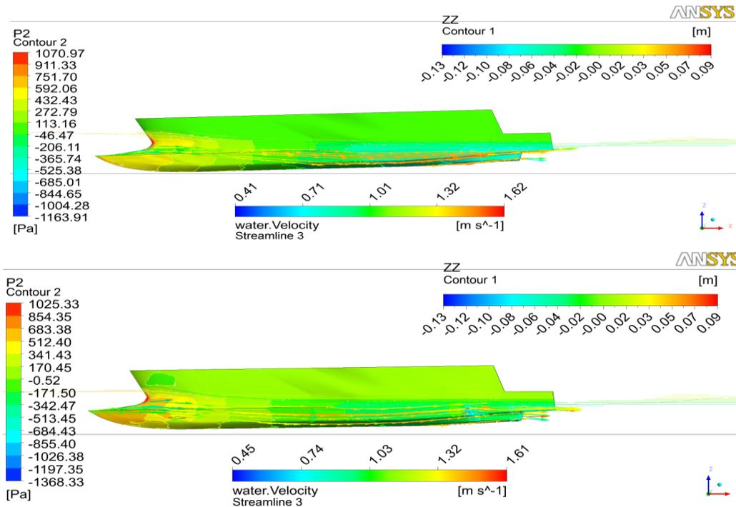
Figure 7: Pressure distribution contour plot of the Semi-SWATH at  $Fr = 0.34$  and  $Fr_H = 1.0$  for the shallow water condition: (top) without fin stabilizers, (bottom) with fin stabilizers ( $\alpha = 0^\circ$ )
