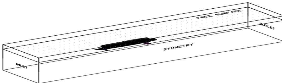
Figure 4: Schematic diagram of the computational domain for the Semi-SWATH hull
