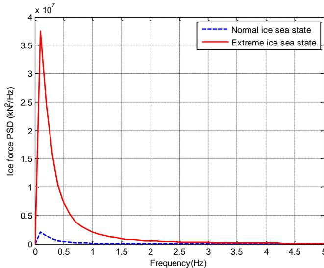
Figure 3: Ice force spectrum for continuous ice crushing under different sea states
