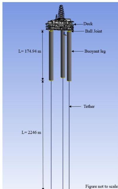
Figure 1: Numerical Model of Triceratops
