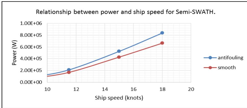
Figure 7: Relationship between power and ship speed for Semi-SWATH
