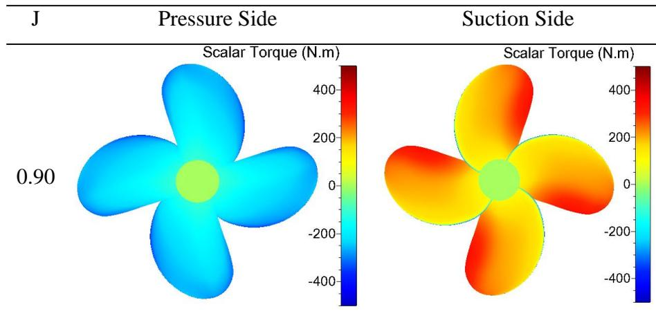
(b) Scalar torque for optimum advance ratio at  $Z=4$ Figure 8: (a)  $Z=3$  and (b)  $Z=4$  Scalar torque on pressure side and suction side
