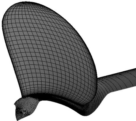
Figure 5: Surface mesh for single blade of propeller.
