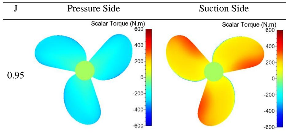
(a) Scalar torque for optimum advance ratio at  $Z=3$ .
