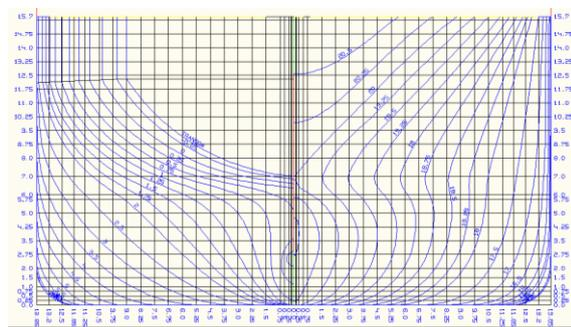
Figure 1. Body Plan of the tanker 17.500 DWT
