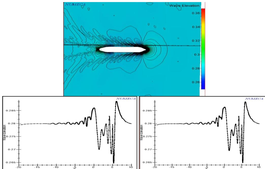
Figure 7. Wave elevation at  $y/L_{pp}=0.148$
