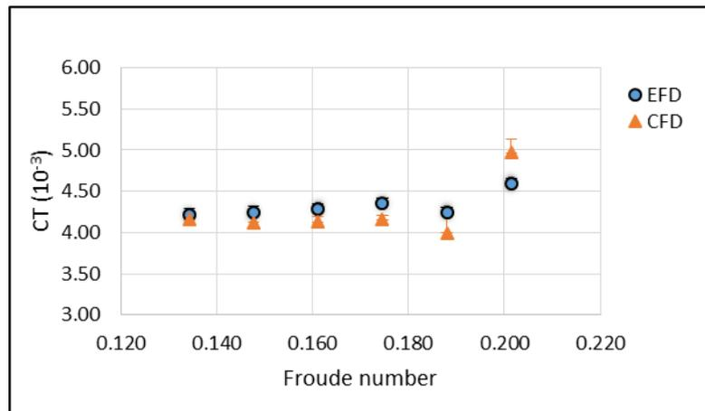
Figure 10. Total resistance coefficient
