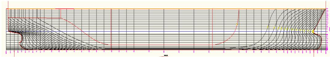
Figure 2. Waterlines of the tanker 17.500 DWT
