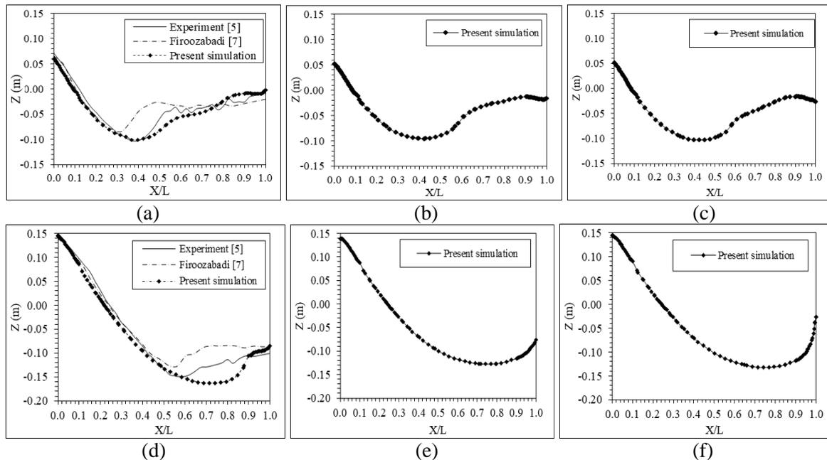
Figure 3: Wave profile for  $Fr = 0.37$  along rudder with (a) NACA 0024 (b) NACA 0012 (c) NACA 0018 foil section, and for 0.55 along (d) NACA 0024 (e) NACA 0012 (f) NACA 0018 foil sections.
