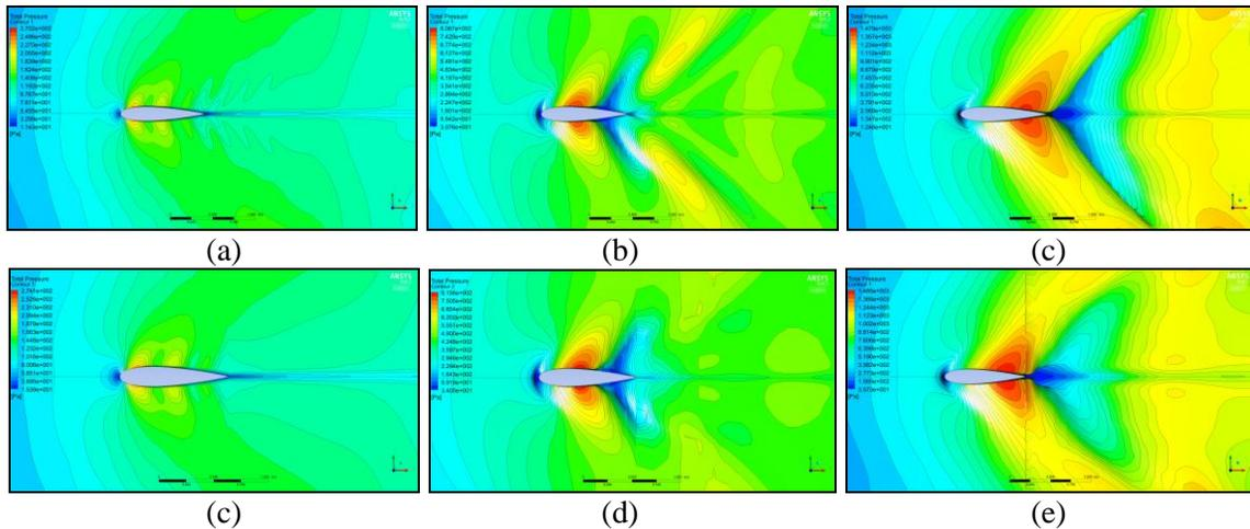
Figure 6: Pressure contours for rudder with NACA 0012 at (a)  $Fr = 0.19$  (b)  $Fr = 0.37$  (c)  $Fr = 0.55$  and for NACA 0018 at (d)  $Fr = 0.19$  (e)  $Fr = 0.37$  and (f)  $Fr = 0.55$ .
