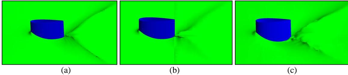
Figure 9: 3D view of free-surface for rudder with (a) NACA 0012 (b) NACA 0018 and (c) NACA 0018 airfoil sections.
