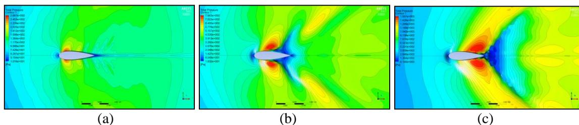
Figure 5: Pressure contours for rudder with NACA 0024 airfoil section at (a)  $Fr = 0.19$  (b)  $Fr = 0.37$  and (c)  $Fr = 0.55$ .
