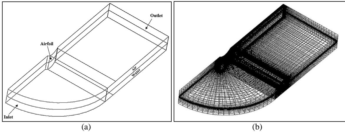
Figure 1: (a) Geometry (b) computational grid for rudder.
