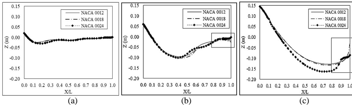
Figure 4: Comparison of the wave profile along different rudder sections at (a)  $Fr = 0.19$  (b)  $Fr = 0.37$  and (c)  $Fr = 0.55$ .
