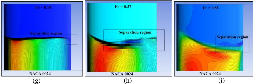
Figure 7: X-wall shear stress contours for rudder with NACA 0012 section at (a)  $Fr = 0.19$  (b)  $Fr = 0.37$  (c)  $Fr = 0.55$ ; with NACA 0018 section at (d)  $Fr = 0.19$  (e)  $Fr = 0.37$  and (f)  $Fr = 0.55$ ; and with NACA 0024 at (g)  $Fr = 0.19$  (h)  $Fr = 0.37$  and (i)  $Fr = 0.55$ .
