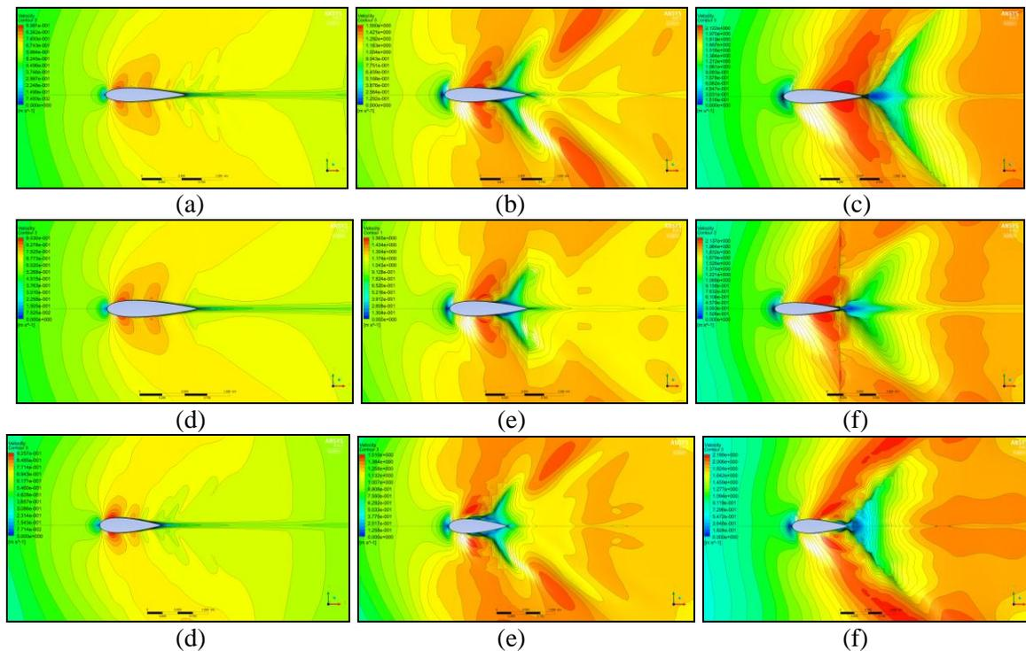
Figure 8: Wave Patterns for rudder with NACA 0012 section at (a)  $Fr = 0.19$  (b)  $Fr = 0.37$  (c)  $Fr = 0.55$ ; with NACA 0018 section at (d)  $Fr = 0.19$  (e)  $Fr = 0.37$  and (f)  $Fr = 0.55$ ; and with NACA 0027 section at (g)  $Fr = 0.19$  (h)  $Fr = 0.37$  and (i)  $Fr = 0.55$ .
