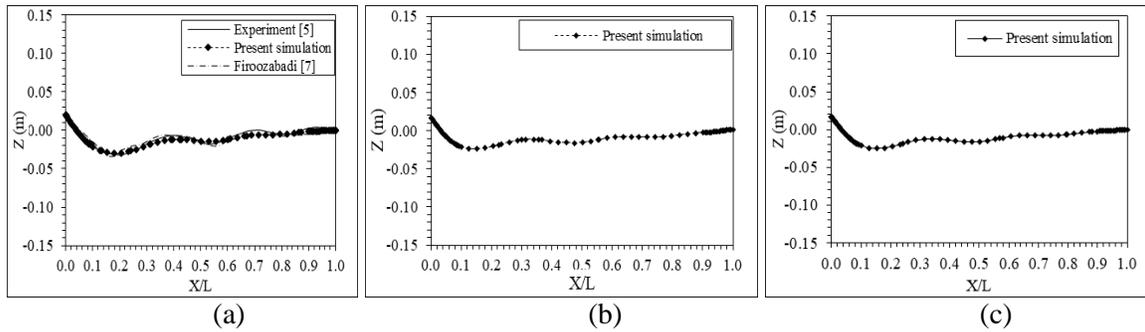
Figure 2: Wave profile for  $Fr = 0.19$  along rudder with (a) NACA 0024 (b) NACA 0012 and (c) NACA 0018 foil sections.
