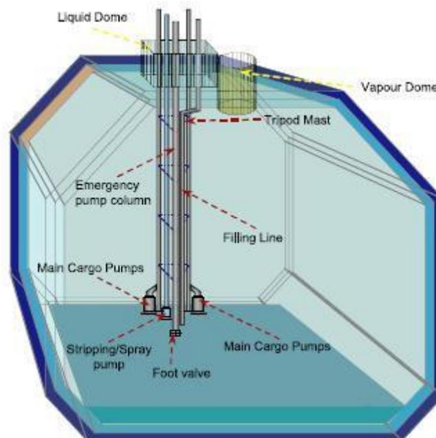
Fig. 5 Pump mast location in membrane tank
