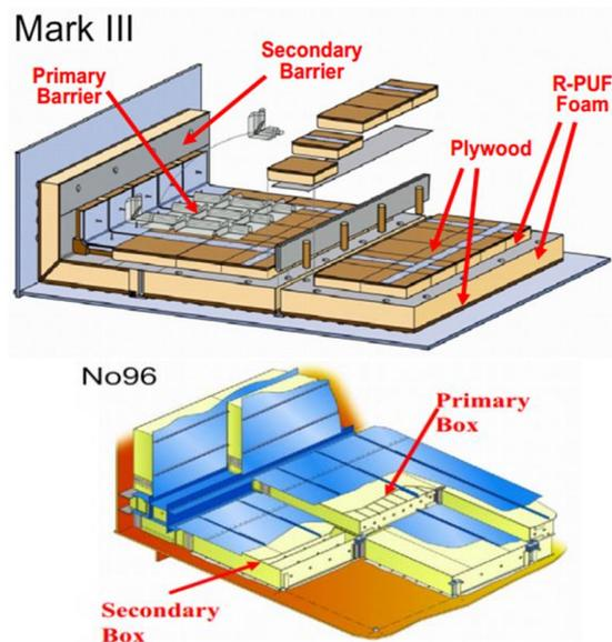
Fig. 3.2 Schematic Drawings of Containment Systems: MARK III and GTT No. 96
