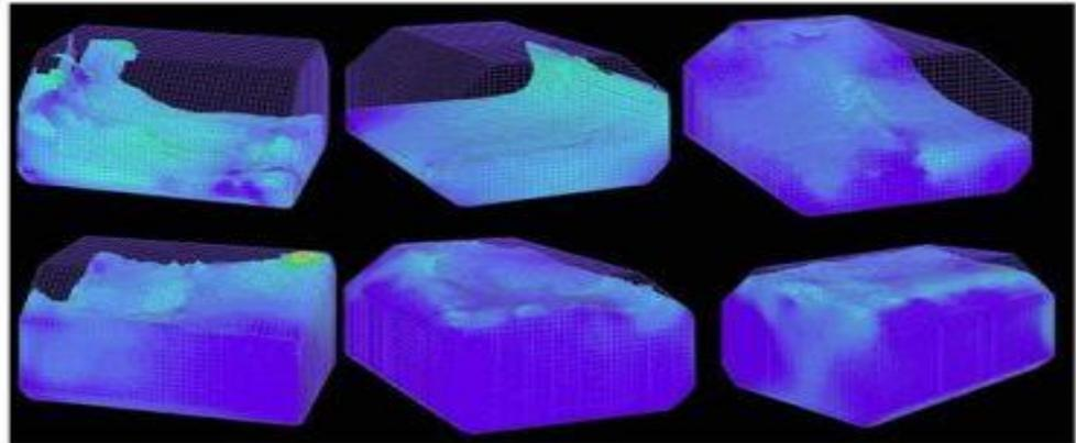
Figure 6.2.1: FLOW-3D® fluid flow animations - Visualisation of impact events for different partial fillings
