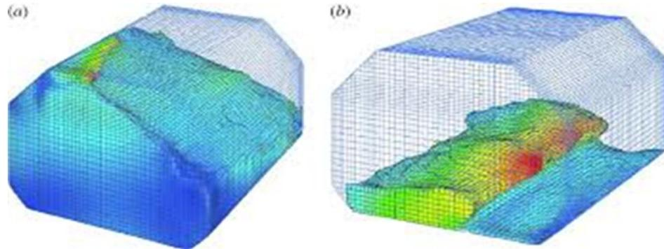
Fig.2 The movement of liquid in LNG tank simulation
