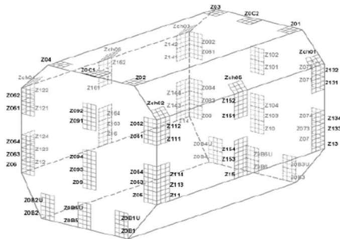
Fig. 6 Default hot spot zones in the membrane tank: Sensors arrangement
