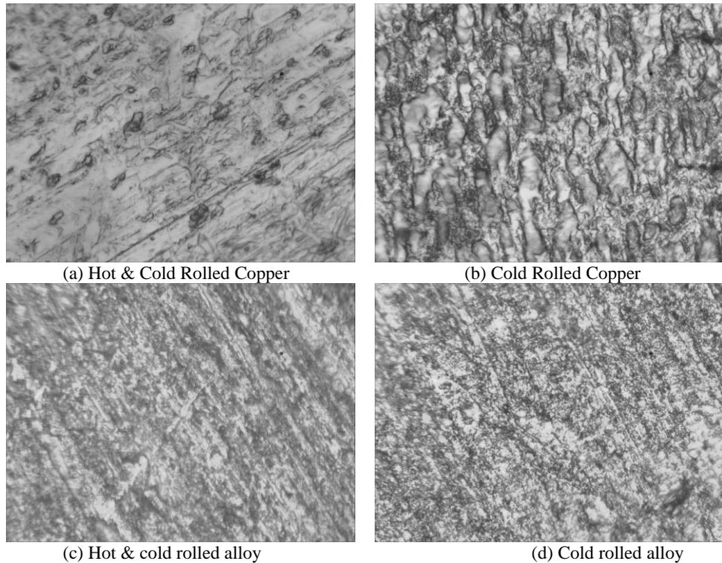
Figure 5: Microstructure of rolled Cu and its alloy at thermal ageing temperature of 400°C with a magnification factor of 1600
