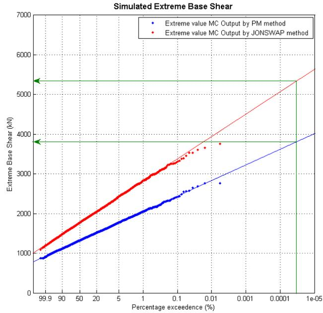
Figure 5: Probability distribution of extreme values using P-M and JONSWAP spectrum for quasi-static base shear  $H_s = 15\text{m}$ ,  $T_z = 13.75\text{sec}$ ,  $U = 0\text{ m/s}$  and  $T = 3.64\text{hrs}$  with number of response records = 10000.
