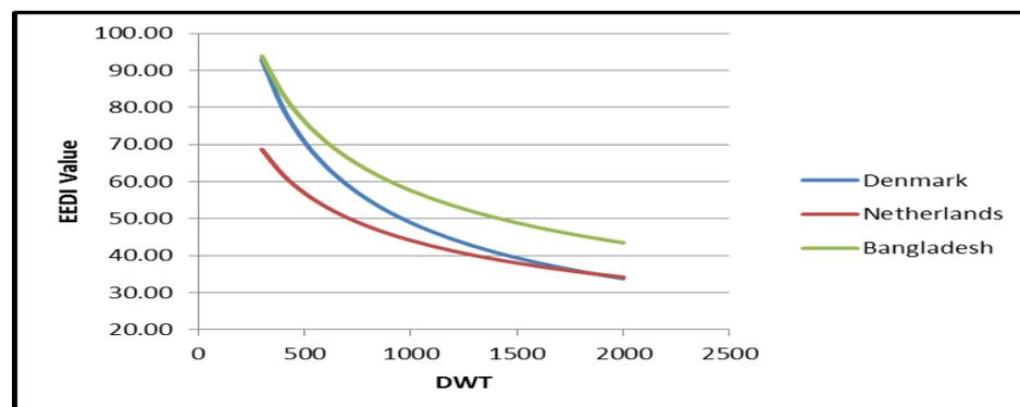
Figure 3: Various countries inland vessels EEDI reference lines for Oil Tanker
