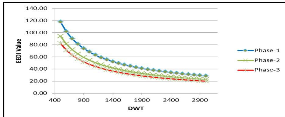
Figure 1: Phase wise EEDI Reference lines for inland Cargo Vessels
