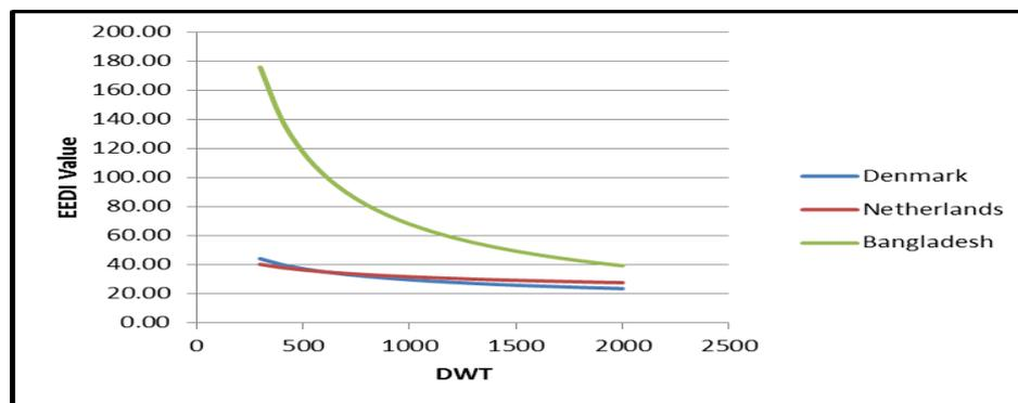
Figure 2: Various countries inland vessels EEDI reference lines for Cargo Vessel
