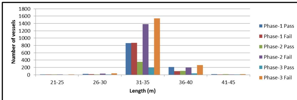
Figure 7: Present status on EEDI with respect to vessel's length for Sand Carrier
