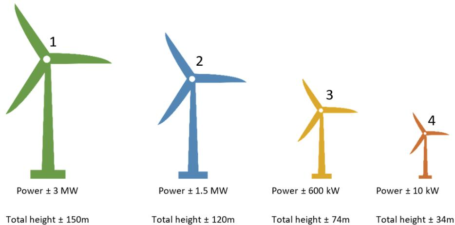
Figure 5: Different scales of wind turbine [14]
