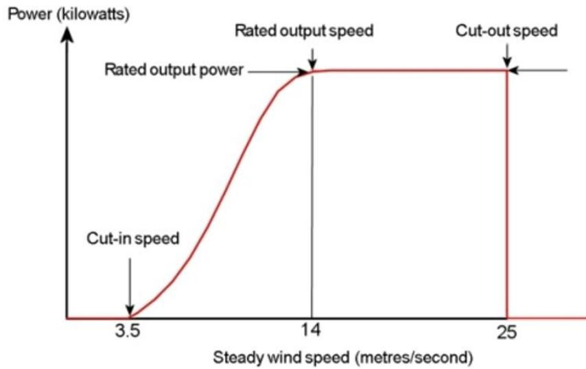
Figure 8: Typical power output for wind turbine depending on the wind speed
