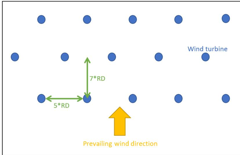
Figure 11: Rows of wind turbines installed according to the rule of thumb
