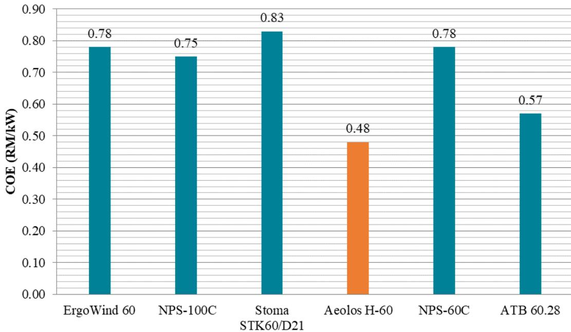
Figure 13: Cost of Energy (COE) by turbine
