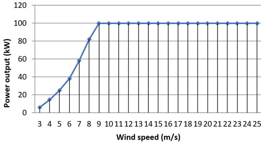
Figure 7: Power curve of the STOMA STK 100kW
