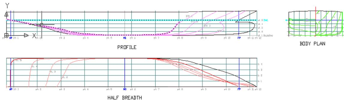
Figure 4: Profile, half breadth and body plan
