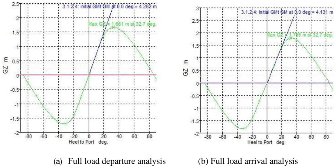
Figure 7: Stability curve for full load departure and arrival
