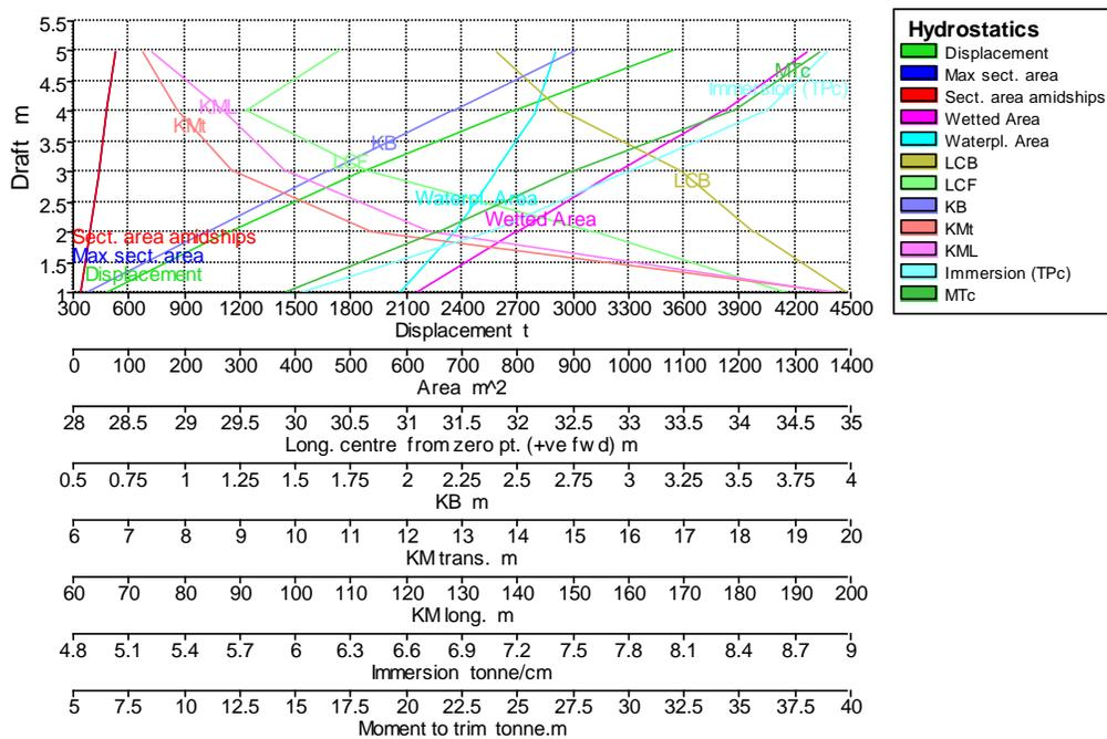
Figure 6: Hydrostatic curves
