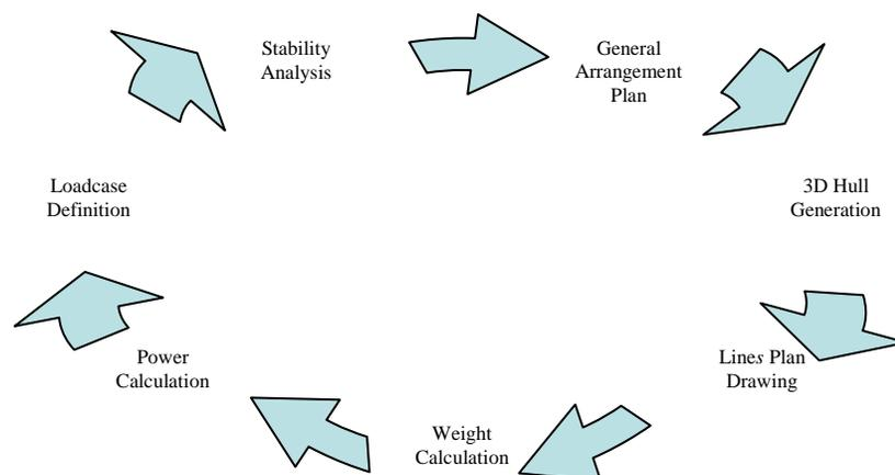
Figure 1: Design spiral for proposed fishing research vessel
