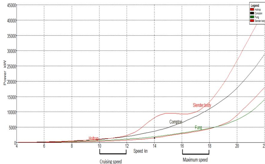
Figure 5: Power vs speed curve
