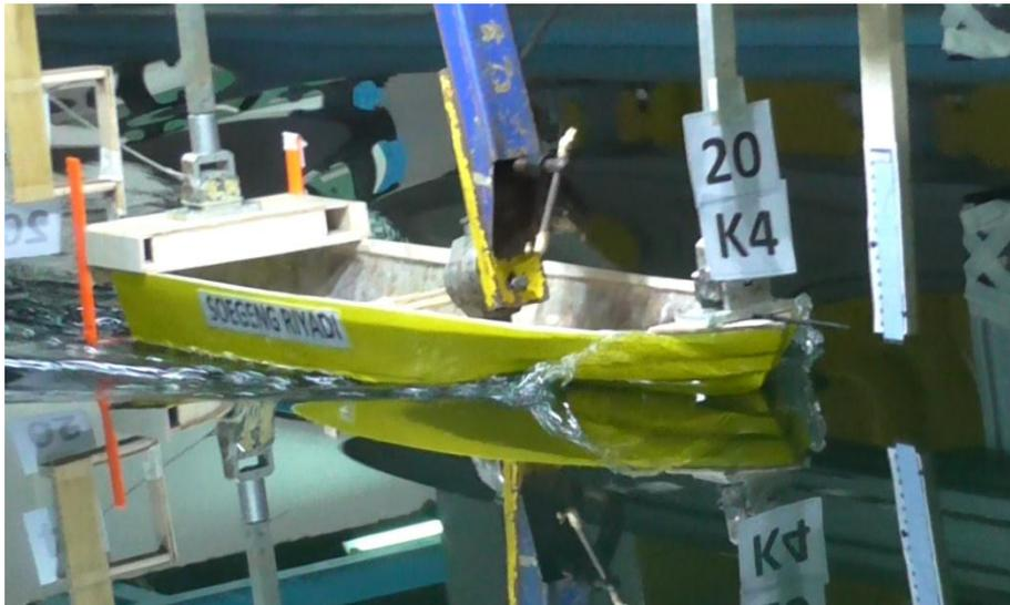
Figure 3: Ship model towed at speed of 1.62 m/s (full-scale speed 20 knot;  $Fr = 0.61$ ).
