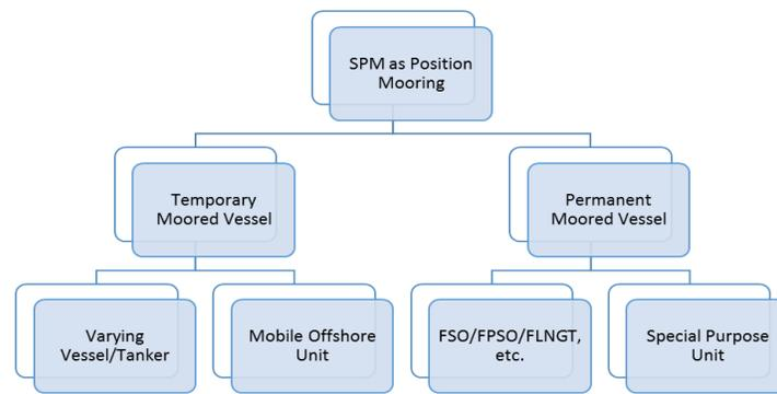
Figure 1: SPM as Position Mooring based on duration of moored vessel
