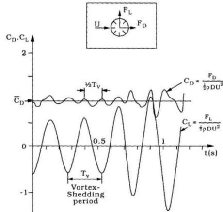
Figure 2: Oscillating drag and lift forces traces, adapted from Sumer
