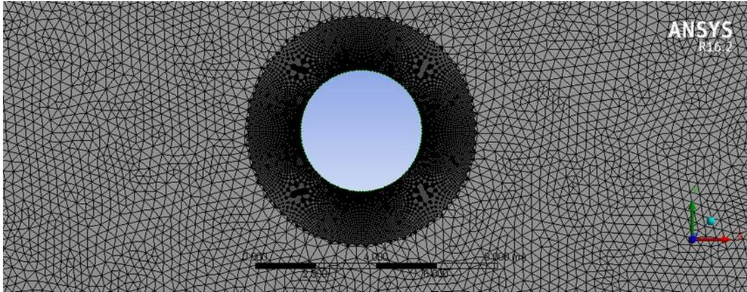
Figure 4: Meshing configuration used ANSYS Fluent.
