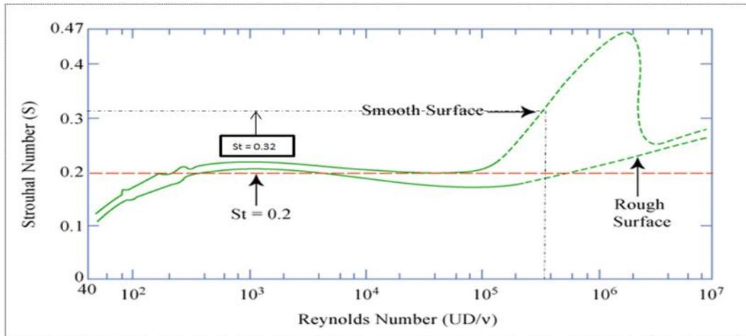
Figure 6: Variation in vortex pattern based on Reynolds number (Re) [4].
