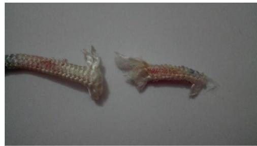
Figure 4: 5mm tested polyester rope sample
