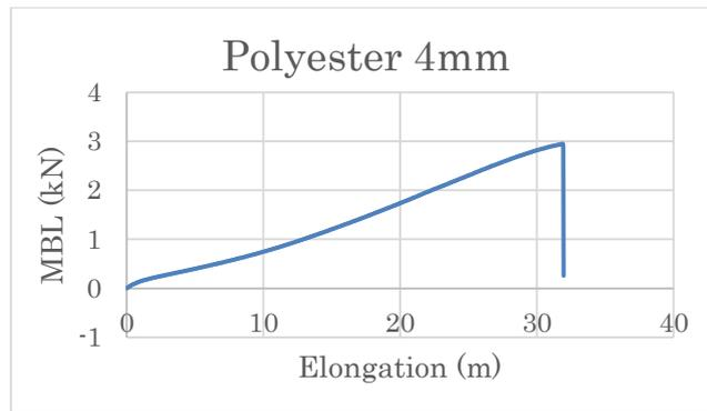
Figure 5: Tensile test result of 4mm nominal diameter polyester rope
