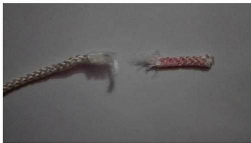
Figure 3: 4mm tested polyester rope sample
