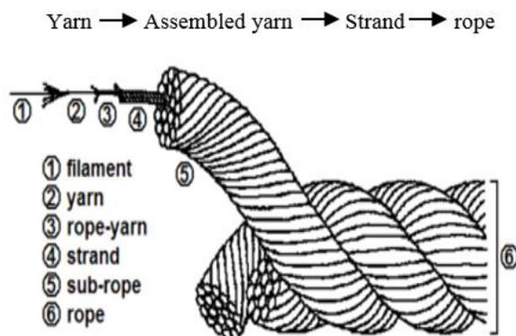
Figure 1: Example of construction geometry of a typical marine synthetic rope (Lechat, Technology, Ecole, & Brest, n.d.)
