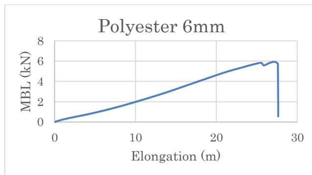
Figure 7: Tensile test result of 6mm nominal diameter polyester rope
