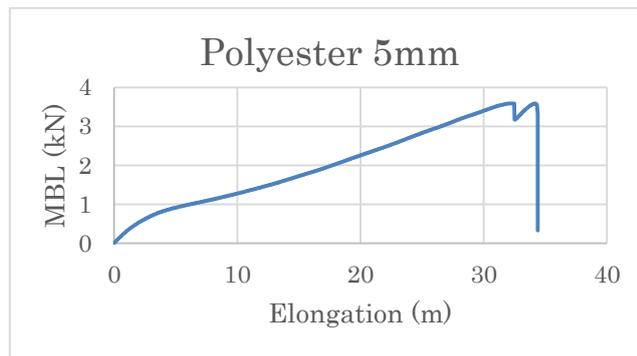
Figure 6: Tensile test result of 5mm nominal diameter polyester rope
