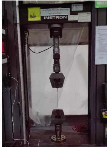
Figure 2: Tensile test machine
