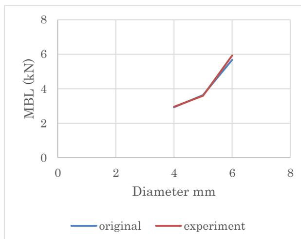
Figure 8: Diameter vs minimum breaking load of polyester rope
